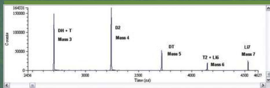
The peaks show the various combinations of D and H molecules. The presence of the peak at mass 5 indicates that there is also Tritium present in the sample. This could however be a more exotic molecule.
