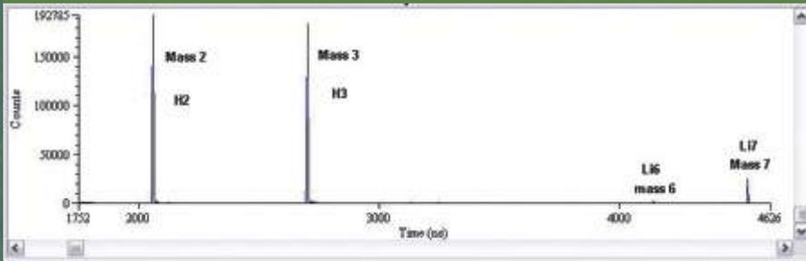
Mass spectrum (in time domain) of the region of a natural water spectrum from about mass 2 to mass 7. The x-axis is flight time in ns.
